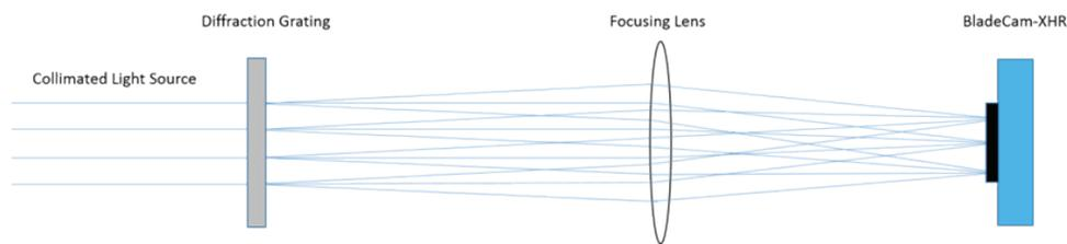
Figure 2 Set-up for Evaluating Performance Diffraction Grating
