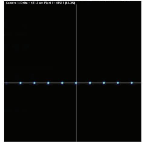
Figure 3 **Diffraction Profile of Beam-splitting Phase Grating**
