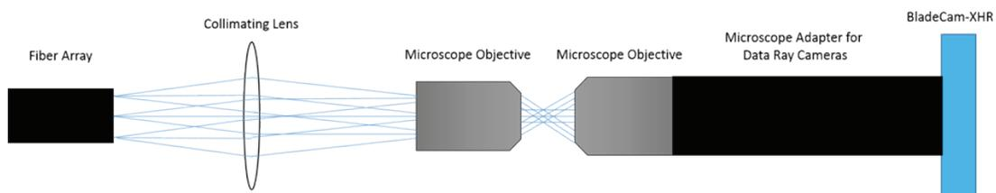
Figure 6 **Setup for Evaluating Performance of Focused 2D Fiber Array**
