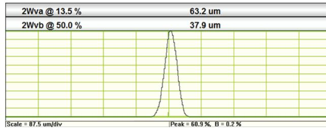
Figure 5 **Vertical profile of the diffracted beam**
