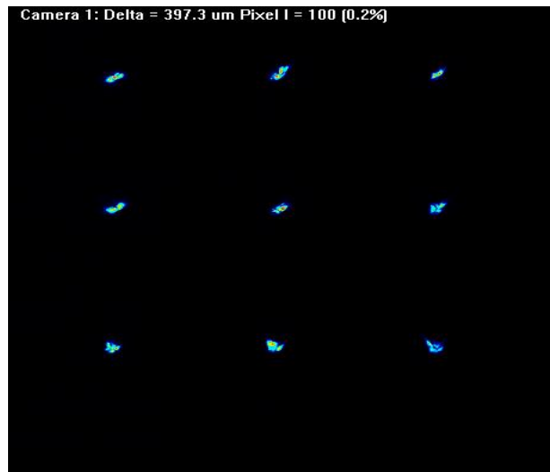
Figure 7 Focused 2D Array of Beams Using Microscope Attachment
