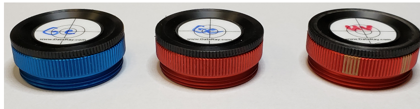
Figure 6: Visual differences between reflective UV and Infrared Filters
