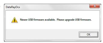
Click OK on the Prompt. The Progress Bar will appear. Programming will take a few tens of seconds. Once it changes to Success etc., disconnect the camera, count to three, reconnect the camera and hit OK.
